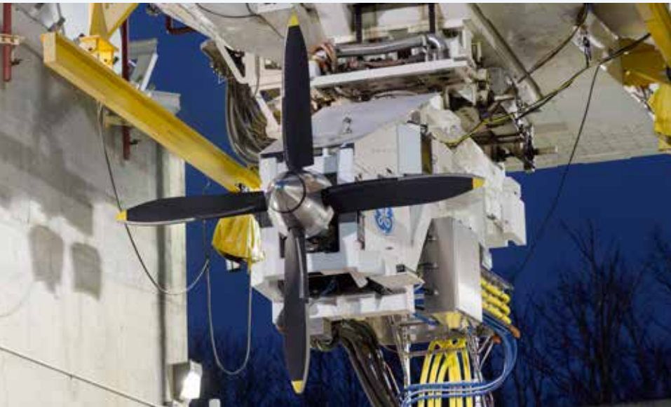
GE Aerospace and NASA recently completed the world's first test of a megawatt (MW)-class and multi-kilovolt (kV) hybrid electric propulsion system. Photo: GE Aerospace
