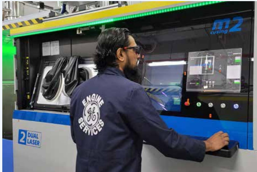
The Loyang facility in Singapore was the first MRO facility worldwide approved to use metal additive manufacturing for commercial jet engine component repairs. Photo: GE Aerospace
