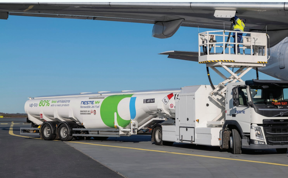
Sustainable Aviation Fuel tanker truck at airport (Photo: Neste)
