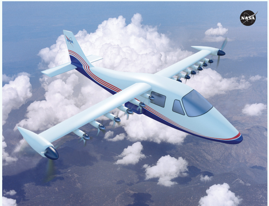
NASA's X-57 Maxwell is an experimental aircraft designed to demonstrate that an all-electric airplane can be more efficient, quieter and more environmentally friendly than airplanes powered by traditional engines (Image: NASA)
